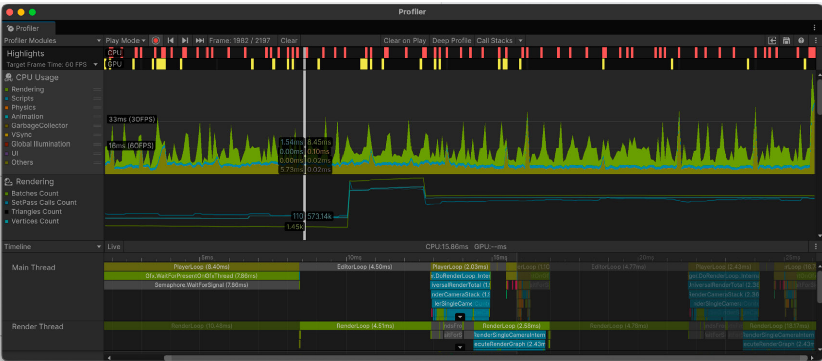
The Timeline view available with the CPU Usage module; this view shows the Main and Render Thread marker detail
