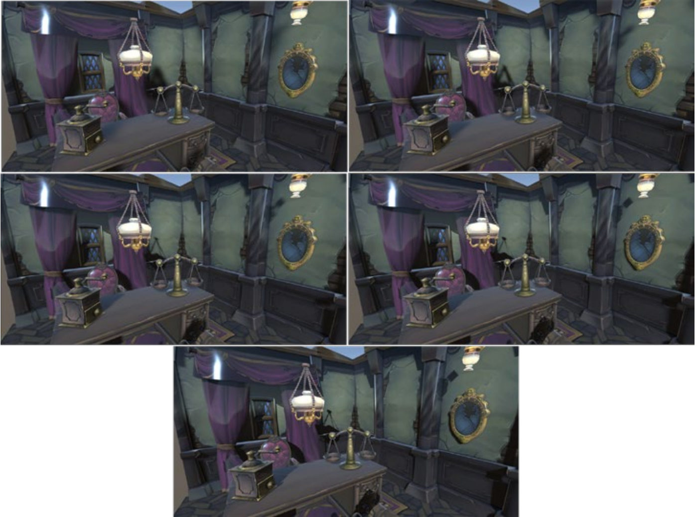
Setting the shadow resolution for the Main Light: The resolution is set to 256 in the top-left image, 512 in the top-right image, 1024 in the middle-left image, 2048 in the middle-right image, and 4096 in the bottom image.
