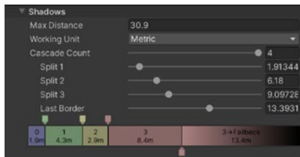
Adjusting the range of a Shadow Cascade
